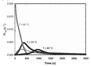
Figure 3. Inferred lumped variable against reaction time for three temperatures: Inferred variable ( $N_{1a}$ ) data from D method step (symbols), and the model predictions ( $N_{1K}$ ) from the ID method result (continuous lines). The initiator concentration is 0.37 mM, initial STY-AN monomer ratio is 1-1, and the assumed initial micelles concentration is  $1 \times 10^{22} \, L^{-1}$ .
