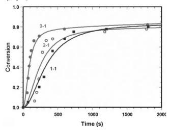
**Figure 6.**Conversion against reaction time for three S-AN initial monomer ratios: Experimental data (symbols) and model predictions from the ID method result (continuous lines). The initiator concentration is 0.37 mM, temperature is 70 °C and the assumed initial micelles concentration is  $1 \times 10^{21}$  (L<sup>-1</sup>).
