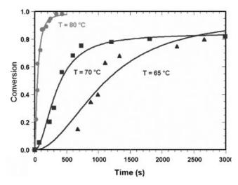
**Figure 4.** Conversion against reaction time for three temperatures: Experimental data (symbols), and the model predictions ID method result (continuous lines). The initiator concentration is  $0.37 \, \text{mM}$ , initial STY-AN monomer ratio is 1-1 and the assumed initial micelles concentration is  $1 \times 10^{21} \, (\text{L}^{-1})$ .
