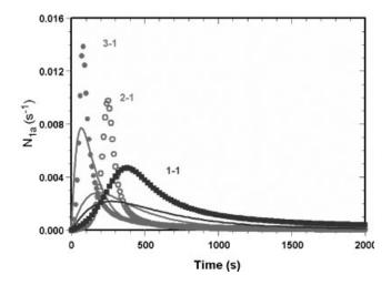
**Figure 5.** Inferred lumped variable (symbols), and model prediction from the ID method result (continuous lines) against reaction time for three initial monomer composition ratios of ST-AN. The initiator concentration is 0.37 mM, and the assumed initial micelles concentration is  $1 \times 10^{22} L^{-1}$ .
