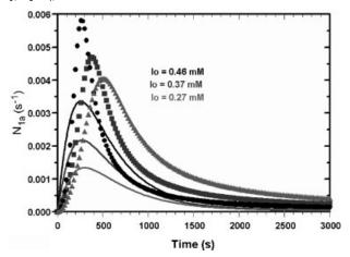
**Figure 1.** Inferred lumped variable against reaction time from the differential (D) method step, for three initiator concentrations. Inferred variable ( $N_{1a}$ ) data (symbols) and the model predictions ( $N_{1k}$ ) from the integrodifferential (ID) method results (continuous lines). The reaction temperature is 70 °C, initial STY-AN monomer composition ratio is 1-1, and the assumed initial micelles concentration is  $1 \times 10^{22} \, L^{-1}$ .
