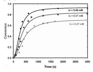
Figure 2. Conversion against reaction time for three initiator concentrations: Experimental data (symbols), and the ID method-based model predictions (continuous lines). The reaction temperature is 70 °C, initial STY-AN monomer ratio is 1-1, and the assumed initial micelles concentration is  $1 \times 10^{21}$  (L<sup>-1</sup>).
